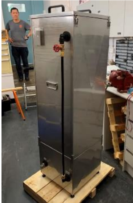
ANSTO 200 L dual-loop two-filter Rn-222 detector
