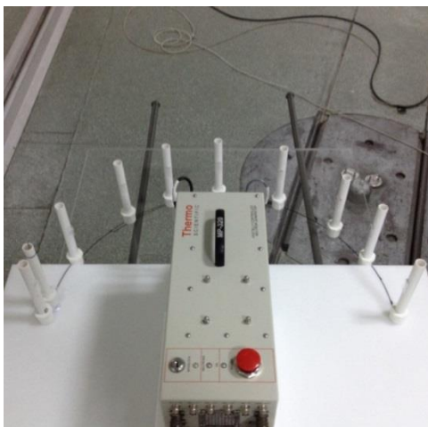
Figure 2. The positioning of CR-39 detectors in the vertical plane surrounding the generator.
